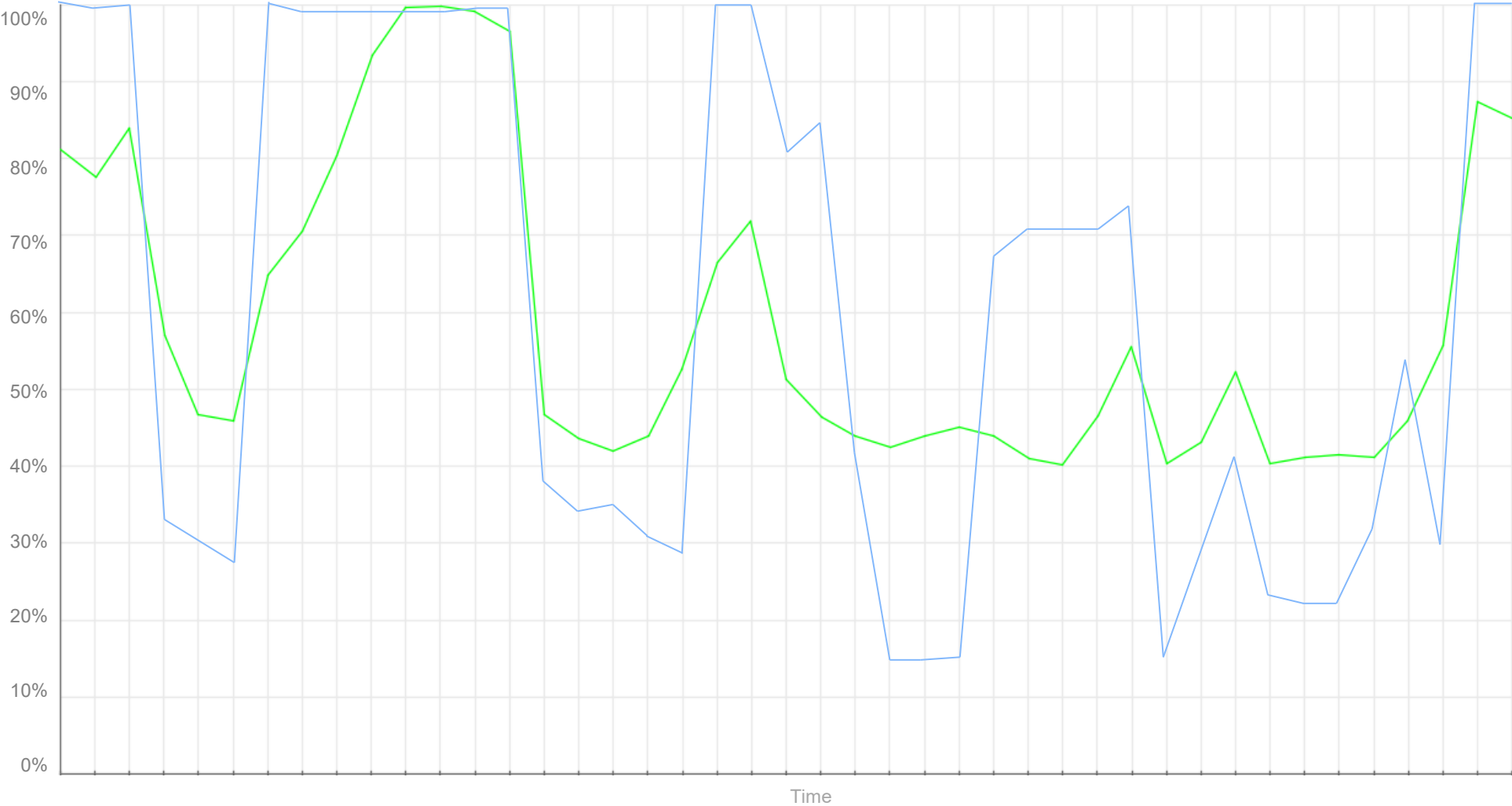
The Power Availability Profile and the Ammonia Capacity Profile (Optimized Variable) for the Optimal Case
