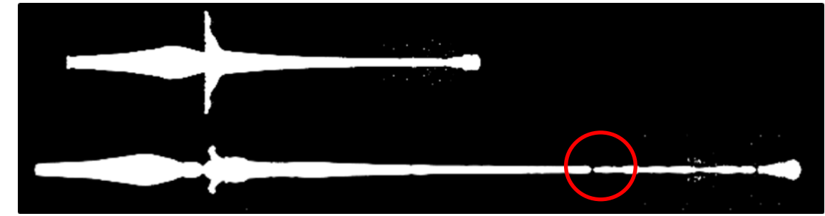
X-ray images of the shaped charge jet at two successive time points (ABSTRAO \gamma SPH 3D simulation, design based on literature). It can be seen that the jet breaks apart at the second time step, resulting in reduced performance.
